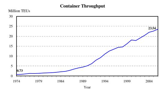
Note: Since there are different sizes of containers, to compile total container throughput, the most commonly used method is to compare the size of each container with that of a twenty-foot standard container (that is 20 ft (length) × 8 ft (width) × 8 ft (height)) in order to covert it into a standard unit for compiling container throughput.
